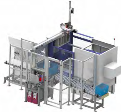
Complete automation cell with crate feeding and IMM by WITTMANN.
